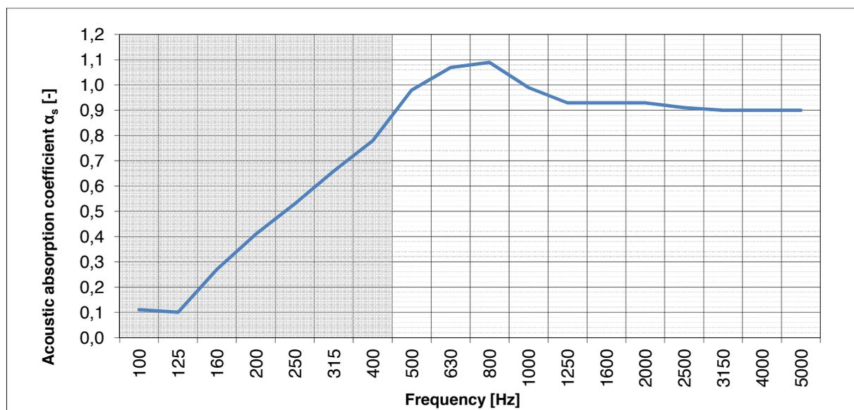
The acoustic absorption coefficients are measured in a reverberation room, according to the ISO 354:2003. The acoustic absorption index  $\alpha_w$  and the acoustic class are evaluated according to the ISO 11654:1998.
